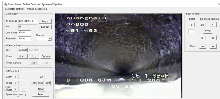
**Figure 5:** Acquisition system interface
