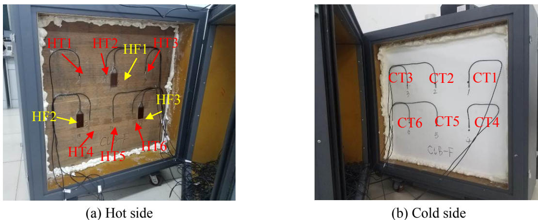
Figure 4: Layout of sensors on the wall
