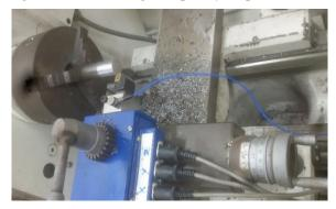
Figure 1 (b): Sensor attached to the tool post
