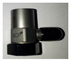
Figure 3: IEPE type Accelerometer
