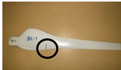
Figure 3b: Blade root crack fault
